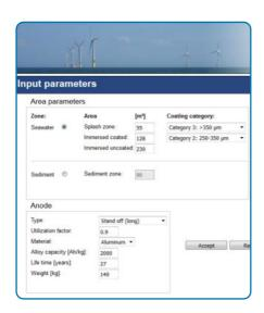
FIELAX developed a web-based application to determine corrosion protection requirements for offshore constructions. Multiple rules and standards were implemented and user-friendly presented. As an alternative to an intranet installation a 'to go' version was setup to be runnable from USB stick.
